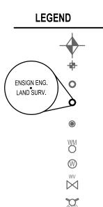
SECTION CORNER MONUMENT EXIST REBAR AND CAP SET ENSIGN REBAR AND CAP SET RIVET WATER METER WATER MANHOLE WATER VALVE FIRE HYDRANT
