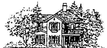
Varied rear-facing slope with some intersecting hip elements Added porch and balcony
