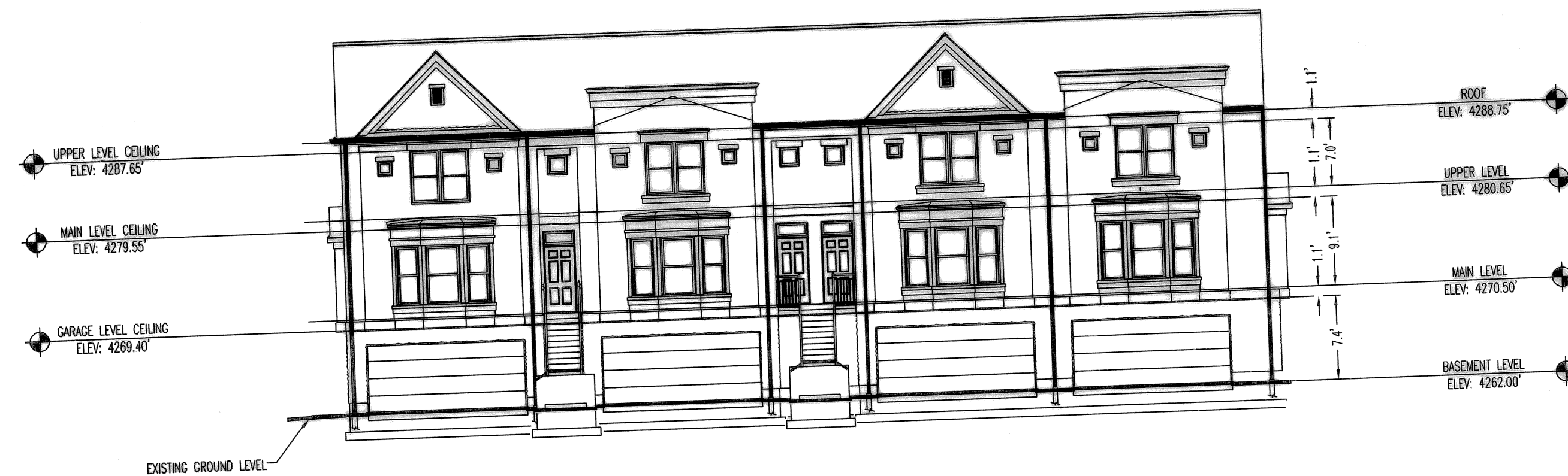
BUILDING "B" FRONT ELEVATION
