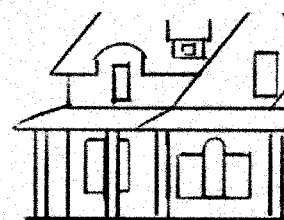
Completely falls apart with multiple roof types, multiple window types, no rhythm for column spacing, competing gables. Elevation studies that have too many dominating elements will not be approved.
