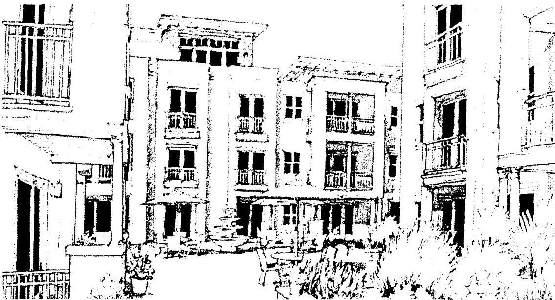
A pedestrian courtyard with apartment buildings. Note that Juliet balconies are employed extensively on the buildings. Also note that an interesting horizon line is created by a fourth story setback and extended eaves that create deep shadows.
