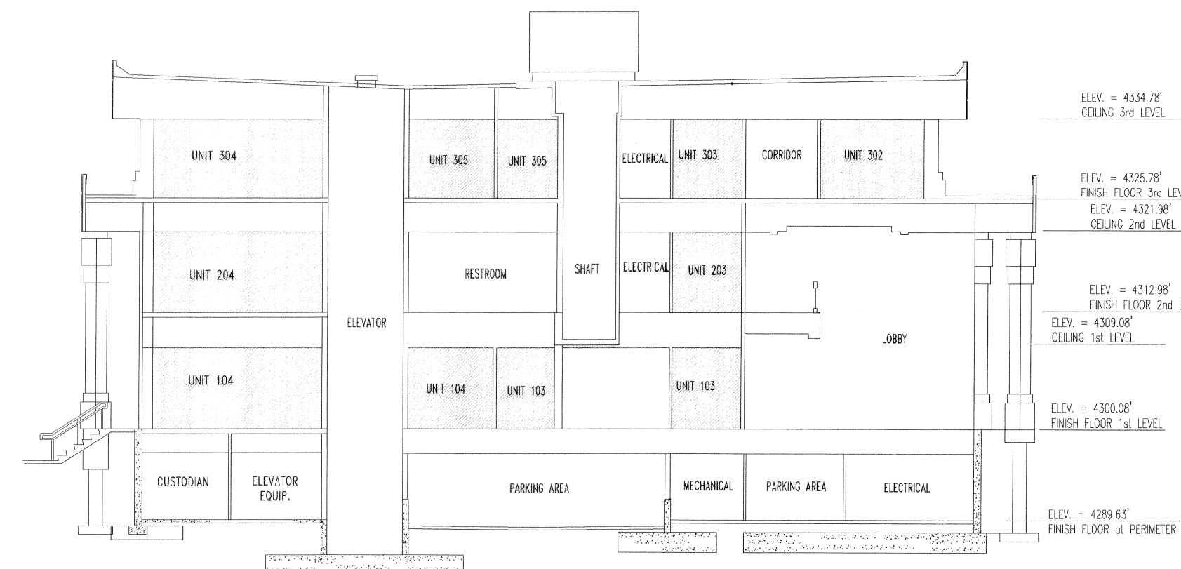
BUILDING CROSS SECTION B
